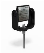
Threaded reference bolts consist of a 3/8'' stainless steel head mounted on a steel rebar (Ø 22 mm) or on an expansion anchor (Ø 14 mm). Supplied with protective plastic cap.
